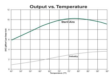
Competitive UVC lights must be changed every 3-4 months to remain effective because their initial output is so low that they quickly lose the intensity or "killing power" needed to maintain biofilm control. The Steril-Aire UVC Emitter, by contrast, has a 12-month service life - and even after a full year, it has greater output than competitive devices deliver on Day 1! As a result, only Steril-Aire can ensure the germicidal performance you need.
