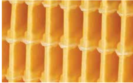
E-Pleat technology molds filtration media into a series of pre-formed channels that direct the air smoothly through the filter, allowing for even loading and complete media utilization.
