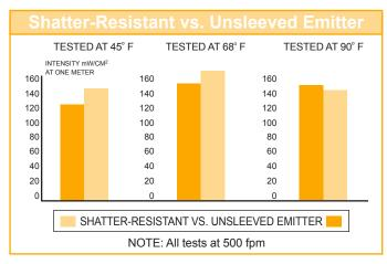
Steril-Aire shatter-proof UVC Emitters provide the highest level of shatter-resistant protection and superior output in the cold conditions typically found in food, beverage and life science applications.
