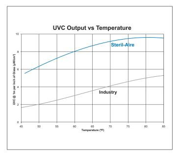
Steril-Aire's multi-patented UVC Emitter provides the best and longest-lasting UVC performance available. As shown in the comparison graph *(above)*, it has been independently tested to deliver up to 6 times the output of other ultraviolet devices under HVAC operating conditions (50 °F @ 400 fpm air velocity).
