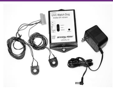
The UVC Watch Dog monitors germicidal UVC Emitter operational status. It is designed to measure change in electrical current to Steril-Aire germicidal UVC Emitter installations and provide Emitter-off status information. Emitter operation status is conveyed with visible LED lights on the mounted Display Unit and/or remote status relayed to a building management system (BMS).
