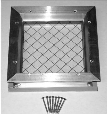
The Steril-Aire AHU Viewport provides a safe, effective means to view working UVC Emitters™ inside an air handling unit (AHU). The AHU Viewport provides installation flexibility for AHU insulated walls of 2" (5.1 cm). It provides the ability to view the interior of the AHU through a 6" x 6" (15.2 cm x 15.2 cm) clear wire glass without the need to open access panels/doors or disconnecting circuits while offering personnel protection against exposure to UVC light.
